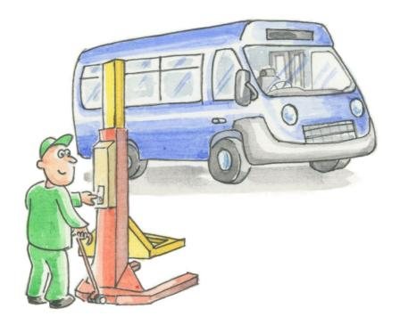
Mobile column lifts are not installed; they are fully mobile, so care must be taken when positioning them. Therefore only correctly trained operators should use and operate these vehicle lifts. Mobile vehicle lifts are available with different lifting capacities and power supplies, i.e. cabled or battery powered.
