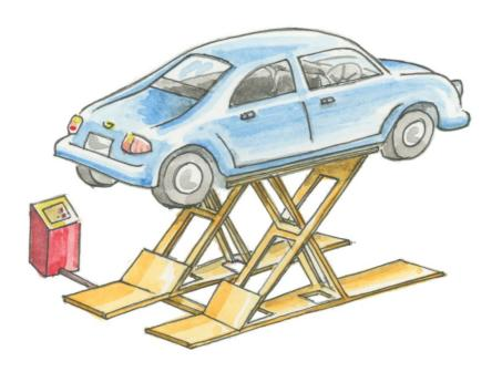
Short platform lifts are designed to lift a vehicle by supporting its chassis, in a similar way to a 2-post lift. However, instead of using arms and pads, a short platform scissor lift utilises 2-platforms on which rubber/plastic lifting blocks are positioned.
