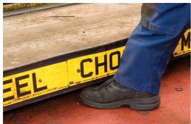
Figure 52 Toe clearance on a vehicle lift
