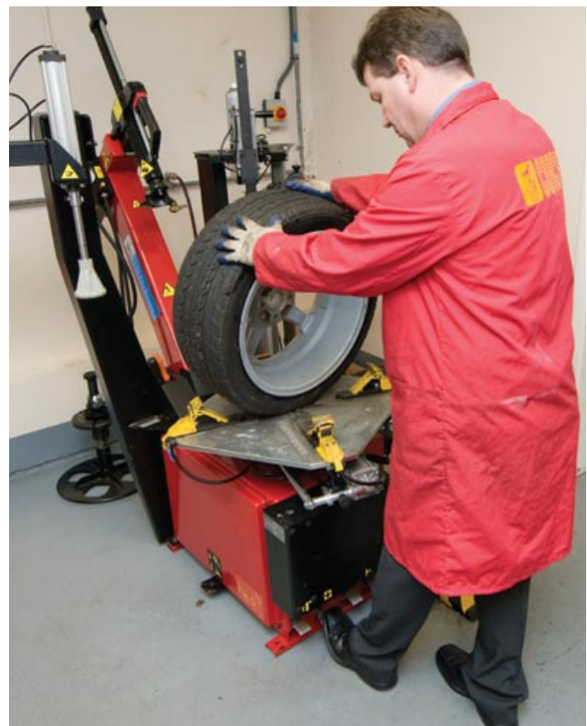
Figure 37 Tyre-changing machine with integrated wheel lift
