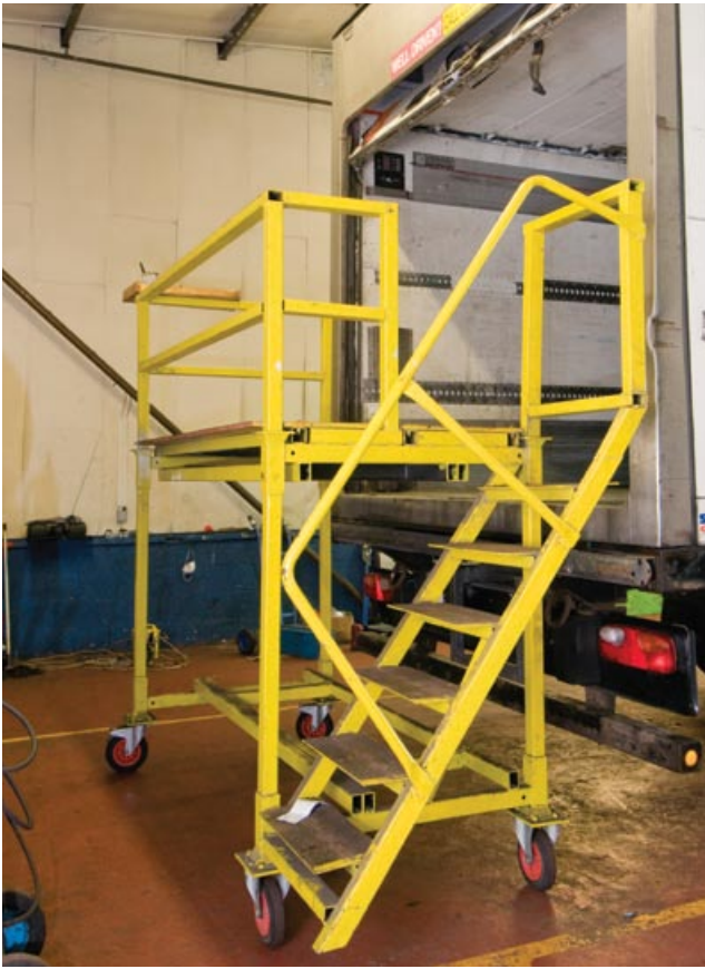
Figure 84 Mobile platform for vehicle access
