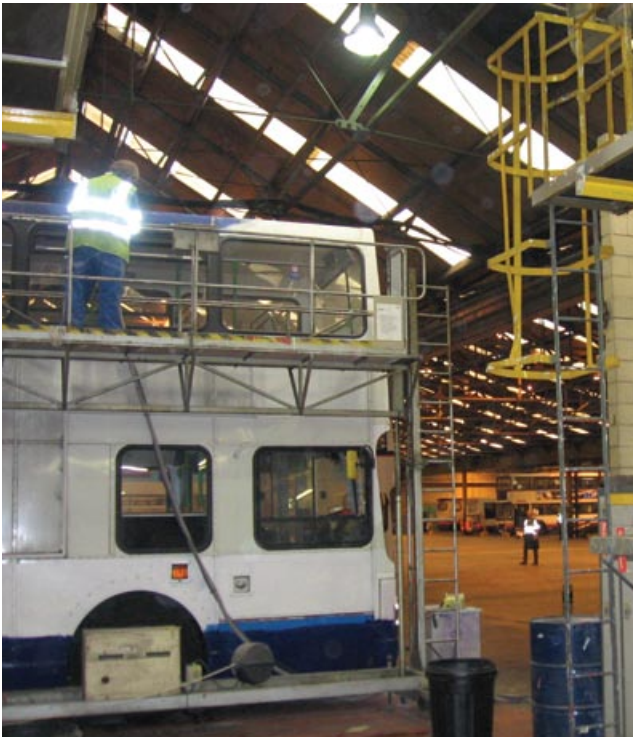
Figure 86 Fixed working platform for buses (photograph courtesy of First Group Plc)
