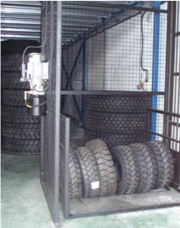
Figure 73 Vertical hoist used for lifting tyres to mezzanine storage (photograph courtesy of Penny Hydraulics Ltd)
