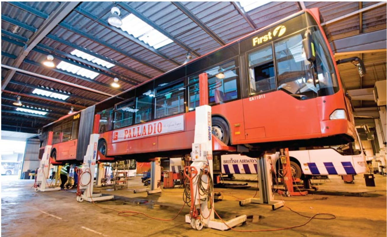
Figure 48 Six-synchronised mobile lifts
