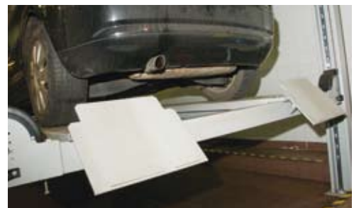
Figure 4 Hinged end-stops help prevent the vehicle falling from the lift when elevated
