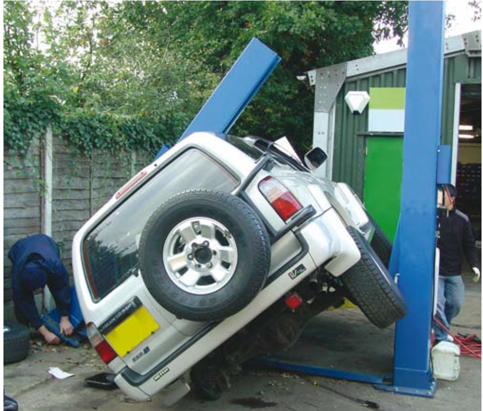
Figure 2 A collapsed two-post lift
