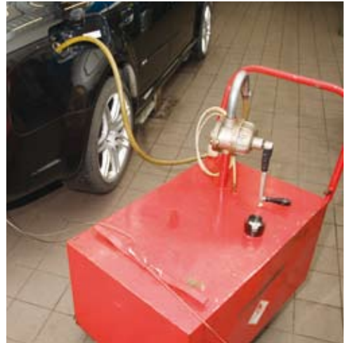
Figure 9 Fuel retriever – note metal collection tank and earthing straps
